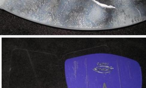
I just built a second fin from the patterns. I had a little problem this time with the router jumping and gouging the patterns leading to a few nicks, but nothing serious. Welding still is bubbly and cloudy, but solid. It's hard to get the pieces clamped in time, welding goes that fast!!! Somehow the footpocket layout is got skewed about 3/8". I'll probably have to do some adjustments on the heel pockets yet.
