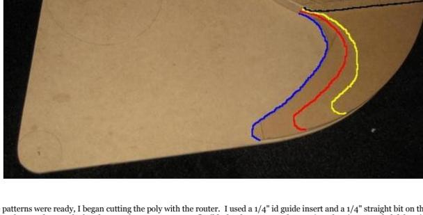
Once the patterns were ready, I began cutting the poly with the router. I used a 1/4" id guide insert and a 1/4" straight bit on the router. I had to cut the top plate on the bandsaw as the pattern was too flexible for the router. After cutting, the pieces needed deburring before welding in place. Some 240 grit sandpaper took care of that. Also sand all interior curves smooth. After sanding strip the protective layers on all pieces and wash them to remove fingerprints and any debris.
