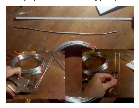
Insert this into the sling, by pushing the tips of each end through holes in the braid that are far towards the edge. Then work the wire through twice more, and bend the wire so it passes through without distorting the sling.
